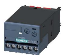
electronic timing relay, ON-delay, with semiconductor output, time range 0.05-100 s, 90-240 V AC/DC, 50/60 Hz, varistor for attenuation of the contactor coils integrated, screw terminal, can be snapped on at the front on contactors 3RT2.3 / 3RT2.4
