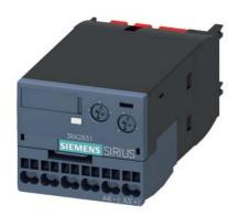
electronic timing relay, ON-delay, with semiconductor output, time range 0.05-100 s, 90-240 V AC/DC, 50/60 Hz, varistor for attenuation of the contactor coils integrated, spring-loaded terminal, can be snapped on at the front on contactors 3RT2.3/3RT2.4
