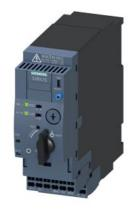
SIRIUS Compact load feeder DOL starter 690 V 110...240 V AC/DC 50...60 Hz 3...12 A IP20 Connection main circuit: plug-in, without terminals Connection auxiliary circuit: Spring-type terminal
