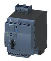
SIRIUS Compact load feeder Reversing starter 690 V 110...240 V AC/DC 50...60 Hz 1...4 A IP20 Connection main circuit: Screw terminal Connection control circuit: screw terminal
