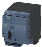
SIRIUS Compact load feeder Reversing starter 690 V 24 V AC/DC 50...60 Hz 0.32...1.25 A IP20 Connection main circuit: plug-in, without terminals Connection control circuit: Spring-type terminal
