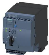
SIRIUS Compact load feeder Reversing starter 690 V 110...240 V AC/DC 50...60 Hz 1...4 A IP20 Connection main circuit: plug-in, without terminals Connection control circuit: Spring-type terminal
