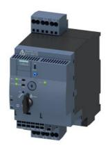
SIRIUS Compact load feeder Reversing starter 400 V 110...240 V AC/DC 50...60 Hz 8...32 A IP20 Connection main circuit: Spring-type terminal Connection control circuit: Spring-type terminal
