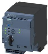
SIRIUS Compact load feeder Reversing starter for IO-Link 400 V 24 V DC 8...32 A IP20 Connection main circuit: plug-in, without terminals Connection control circuit: Spring-type terminal
