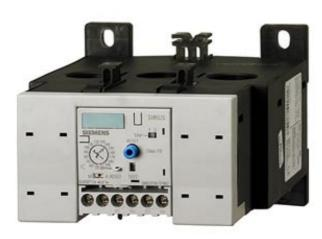
OVERLOAD RELAY 50...200 A FOR MOTOR PROTECTION SIZE S6, CLASS 10 MOUNT. ONTO CONT./ STAND-ALONE MAIN CIRCUIT: BAR CONNECTION AUX. CIRCUIT: SCREW CONNECTION MANUAL-AUTOMATIC-RESET
