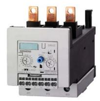
Overload relay 25...100 A For motor protection Size S3, Class 5...30 Contactor mounting Main circuit: Screw terminal Auxiliary circuit: Spring-type terminal Manual-Automatic-Reset Internal ground fault detection !!! Phased-out product !!! Successor is SIRIUS 3RB3 Preferred successor type is >>3RB3143-4XD0<<
