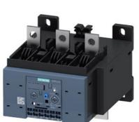
Overload relay 50...200 A for motor protection Size S6, CLASS 5...30E Contactor mounting/stand-alone installation Main circuit: busbar connection Auxiliary circuit: Spring-type terminal Manual-Automatic-Reset Internal ground fault detection
