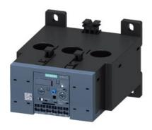
Overload relay 50...200 A for motor protection Size S6, CLASS 5...30E Contactor mounting/stand-alone installation Main circuit: straight-through transformer Auxiliary circuit: Spring-type terminal Manual-Automatic-Reset Internal ground fault detection
