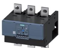
Overload relay 55...250 A for motor protection Size S10/S12, CLASS 5...30E Contactor mounting/stand-alone installation Main circuit: busbar connection Auxiliary circuit: Screw terminal Manual-Automatic-Reset Internal ground fault detection
