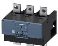
Overload relay 160...630 A for motor protection Size S10/S12, CLASS 5...30E Contactor mounting/stand-alone installation Main circuit: busbar connection Auxiliary circuit: Spring-type terminal Manual-Automatic-Reset Internal ground fault detection
