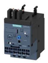
Overload relay 0.1...0.4 A Electronic For motor protection Size S00, Class 10E Contactor mounting Main circuit: Spring-type terminal Auxiliary circuit: Spring-type terminal Manual-Automatic-Reset
