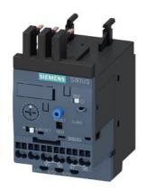
Overload relay 4...16 A Electronic For motor protection Size S00, Class 10E Contactor mounting Main circuit: Spring-type terminal Auxiliary circuit: Spring-type terminal Manual-Automatic-Reset
