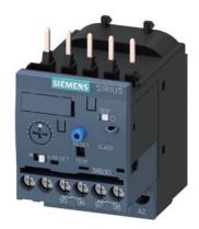
Overload relay 0.32...1.25 A Electronic For motor protection Size S00, Class 20E Contactor mounting Main circuit: Screw Auxiliary circuit: Screw Manual-Automatic-Reset
