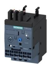
Overload relay 0.32...1.25 A Electronic For motor protection Size S00, Class 20E Contactor mounting Main circuit: Spring-type terminal Auxiliary circuit: Spring-type terminal Manual-Automatic-Reset
