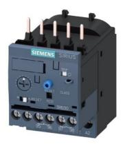
Overload relay 4...16 A Electronic For motor protection Size S00, Class 20E Contactor mounting Main circuit: Screw Auxiliary circuit: Screw Manual-Automatic-Reset
