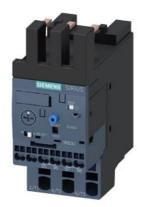
Overload relay 1...4 A Electronic For motor protection Size S0, Class 10E Contactor mounting Main circuit: Spring-type terminal Auxiliary circuit: Spring-type terminal Manual-Automatic-Reset
