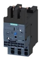
Overload relay 0.1...0.4 A Electronic For motor protection Size S0, Class 10E Contactor mounting Main circuit: Spring-type terminal Auxiliary circuit: Spring-type terminal Manual-Automatic-Reset
