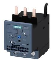
Overload relay 12.5...50 A Electronic For motor protection Size S2, Class 10E Contactor mounting Main circuit: Screw Auxiliary circuit: Spring-type terminal Manual-Automatic-Reset
