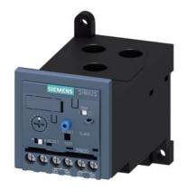
Overload relay 12.5...50 A Electronic For motor protection Size S2, Class 10E Stand-alone installation Main circuit: Straight-through transformer Auxiliary circuit: Screw Manual-Automatic-Reset
