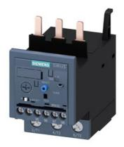
Overload relay 20...80 A Electronic For motor protection Size S2, Class 20E Contactor mounting Main circuit: Screw Auxiliary circuit: Screw Manual-Automatic-Reset
