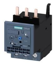
Overload relay 20...80 A Electronic For motor protection Size S2, Class 20E Contactor mounting Main circuit: Screw Auxiliary circuit: Spring-type terminal Manual-Automatic-Reset
