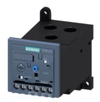
Overload relay 20...80 A Electronic For motor protection Size S2, Class 20E Stand-alone installation Main circuit: Straight-through transformer Auxiliary circuit: Screw Manual-Automatic-Reset
