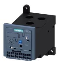
Overload relay 20...80 A Electronic For motor protection Size S2, Class 20E Stand-alone installation Main circuit: Straight-through transformer Auxiliary circuit: Spring-type terminal Manual-Automatic-Reset
