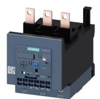
Overload relay 32...115 A Electronic For motor protection Size S3, Class 10E Contactor mounting Main circuit: Screw Auxiliary circuit: Spring-type terminal Manual-Automatic-Reset
