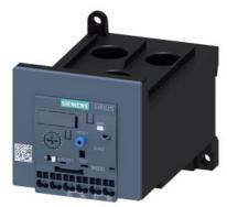
Overload relay 32...115 A Electronic For motor protection Size S3, Class 10E Stand-alone installation Main circuit: Straight-through transformer Auxiliary circuit: Spring-type terminal Manual-Automatic-Reset
