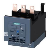
Overload relay 12.5...50 A Electronic For motor protection Size S3, Class 20E Contactor mounting Main circuit: Screw Auxiliary circuit: Spring-type terminal Manual-Automatic-Reset
