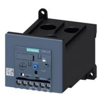
Overload relay 12.5...50 A Electronic For motor protection Size S3, Class 20E Stand-alone installation Main circuit: Straight-through transformer Auxiliary circuit: Screw Manual-Automatic-Reset
