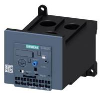
Overload relay 12.5...50 A Electronic For motor protection Size S3, Class 20E Stand-alone installation Main circuit: Straight-through transformer Auxiliary circuit: Spring-type terminal Manual-Automatic-Reset
