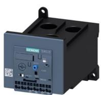
Overload relay 32...115 A Electronic For motor protection Size S3, Class 20E Stand-alone installation Main circuit: Straight-through transformer Auxiliary circuit: Spring-type terminal Manual-Automatic-Reset
