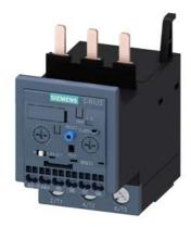
Overload relay 20...80 A Electronic For motor protection Size S2, Class 5E...30E Contactor mounting Main circuit: Screw Auxiliary circuit: Spring-type terminal Manual-Automatic-Reset Internal ground fault detection
