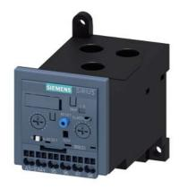
Overload relay 20...80 A Electronic For motor protection Size S2, Class 5E...30E Stand-alone installation Main circuit: Straight-through transformer Auxiliary circuit: Spring-type terminal Manual-Automatic-Reset Internal ground fault detection
