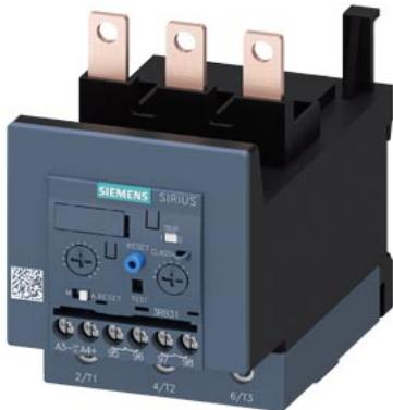
Overload relay 12.5...50 A Electronic For motor protection Size S3, Class 5E...30E Contactor mounting Main circuit: Screw Auxiliary circuit: Screw Manual-Automatic-Reset
