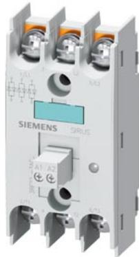
Semiconductor relay, 3-phase 3RF2 30 A / 40 °C 48-600 V / 4-30 V DC 3-phase controlled Ring cable connection Blocking voltage 1200 V
