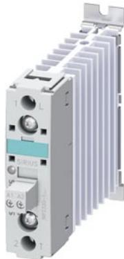
Solid-state contactor 1-phase 3RF2 AC 51 / 20 A / 40 °C 24-230 V / 110-230 V AC screw terminal
