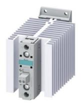
Solid-state contactor 1-phase 3RF2 AC 51 / 50 A / 40 °C 24-230 V / 110-230 V AC screw terminal
