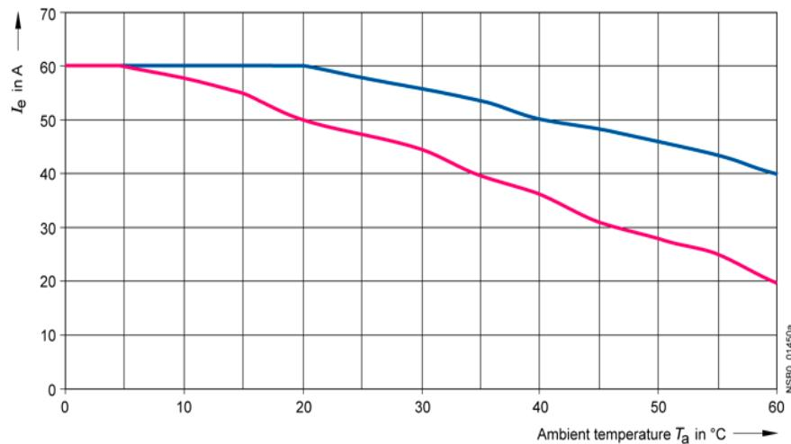
—  $I_{\max}$  Thermal limit current for individual and side-by-side mounting
