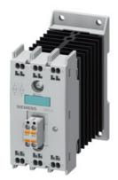
Solid-state contactor 3-phase 3RF2 AC 51 / 20 A / 40  $^{\circ}$ C 48-600 V / 4-30 V DC 2-phase controlled Spring-type terminal Blocking voltage 1200 V
