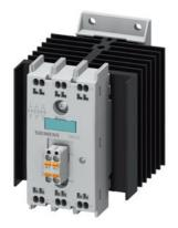
Solid-state contactor 3-phase 3RF2 AC 51 / 20 A / 40  $^{\circ}$ C 48-600 V / 4-30 V DC 3-phase controlled Spring-type terminal Blocking voltage 1200 V
