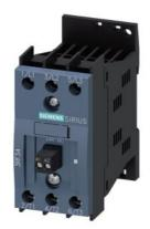
Solid-state contactor 3-phase 3RF3 AC 53 / 5.2 A / 40  $^{\circ}$ C 48-480 V / 24 V DC 2-phase controlled Instantaneous switching screw terminal
