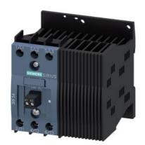
Solid-state contactor 3-phase 3RF3 AC 53 / 9.2 A / 40  $^{\circ}$ C 48-480 V / 110-230 V AC 2-phase controlled Instantaneous switching screw terminal
