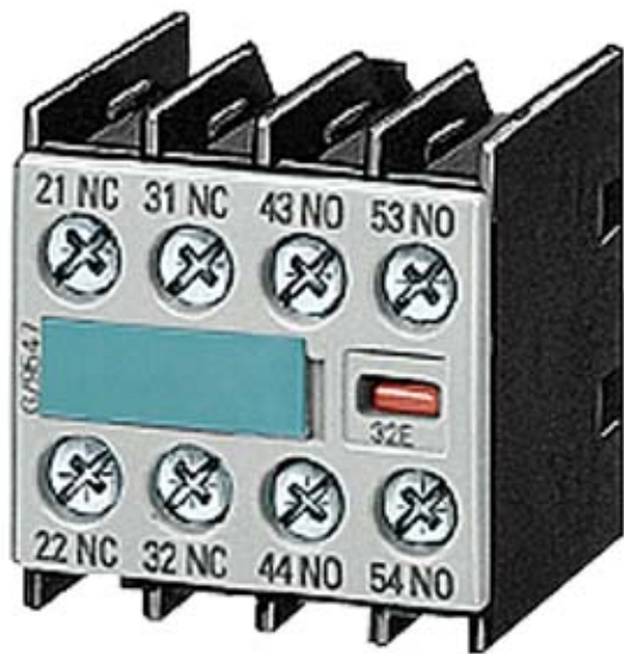
AUXILIARY SWITCH BLOCK, 32E, 2NO+2NC, DIN EN50012, SCREW CONNECTION, FOR CONTACTORS FOR SWITCHING MOTORS, 4-POLE
