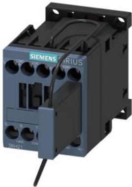
Contactor relay railway, 2 NO + 1 NC 125 V DC, 0.7 ... 1.25\* US, with integrated suppressor diode, Size S00, screw terminal installation on standard mounting rail optimized (20 G) suitable for PLC outputs
