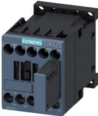
Coupling contactor relay, 2 NO + 2 NC, 24 V DC, 0.85 ... 1.85\* US, with varistor plugged on, Size S00, screw terminal
