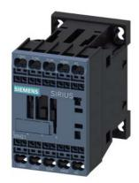
Contactor relay, 2 NO + 2 NC, 110 V AC, 50 Hz, 120 V, 60 Hz, Size S00, Spring-type terminal
