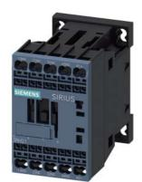
Coupling contactor relay, 2 NO + 2 NC, 24 V DC, 0.7 ... 1.25\* US, with integrated diode, Size S00, Spring-type terminal suitable for PLC outputs
