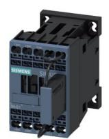
Contactor relay for railway, 2 NO + 1 NC, 24 V DC, 0.7 ... 1.25\* US, with integrated suppressor diode, Size S00, Spring-type terminal suitable for PLC outputs
